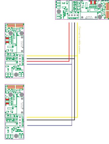
Note: When using RS-232 interfaces only one Mini-Rep will be able to control the Orion conventional panel. All other Orion Mini-Rep's will only be able to displaysystem status.
